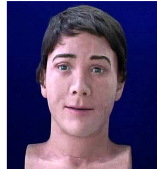
Fig. 4. The employed robot head ‘Jules’ has 34 servo motors emulating the majority of the human facial muscles in face and neck.
